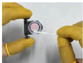
4. Use a dust-free cotton swab dipped in alcohol or a dust-free cloth to gently wipe the front of the protective lens
