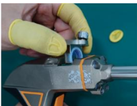
2. Take out the protective mirror base
