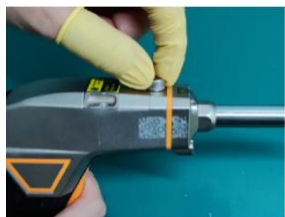
1. Unscrew the protective mirror seat screw
