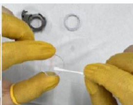
5. Take out the protective mirror fixing piece for protection Wipe the other side of the goggles
