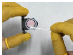
4. Use a dust-free cotton swab dipped in alcohol or a dust-free cloth to gently wipe the front of the protective lens
