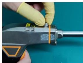
1. Unscrew the protective mirror seat screw
